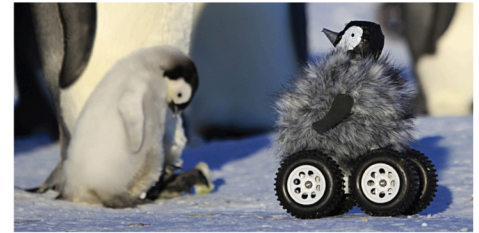
Polar biology: Field work using a rover camouflaged with an emperor penguin chick model “huddling” with chicks in a crèche. The rover was able to infiltrate the emperor penguin crèche without disturbance, thus demonstrating the possibility to use such a camouflaged rover to collect data from locations within a colony that are not accessible to a human investigator. Picture by Frédérique Olivier © John Downer Production
